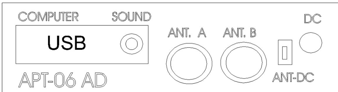
The **APT-06** has no power on-off switch. As soon as power is plugged in, it will power up and the 5 red LEDs start blinking all together for about 5 seconds.
