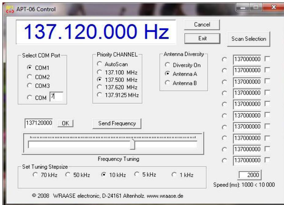
**APT-CONTROL** offers several frequency selection options: While in the field „Priority-Channel“ the fixed channels within the **APT-06** firmware are selected, the other frequency control options directly access the **APT-06** digital synthesizer
